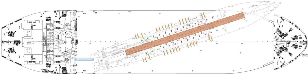
*Final topside arrangement showing locations of keel blocks, side blocks, spur shores, and access/service brow*
