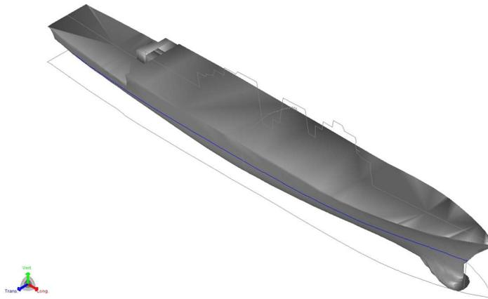
*3D view of target cargo (Flight III Arleigh Burke class destroyer) POSSE model*
