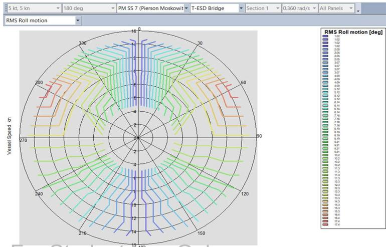
*Roll motion for loaded heavy lift vessel in Sea State 7 (17.4 degree max roll angle)*
