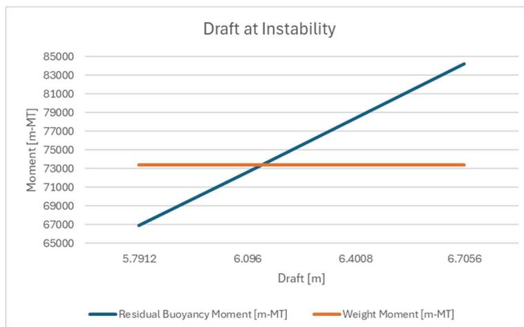
The target cargo's draft at instability is graphically represented by the point where the residual buoyancy moment and weight moment are equal.
