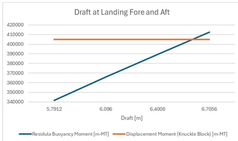
*The target cargo's draft at landing forward and aft is graphically represented by the point where the residual buoyancy moment and displacement moment about the knuckle block are equal.*
