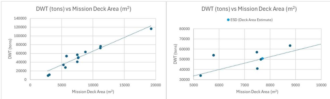
*Scatter plots of heavy lift vessels used to interpolate Montford Point's DWT*
