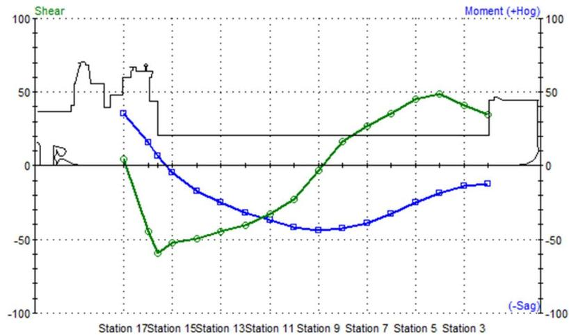
*9 m submergence percent allowable shear and moment with distributed ballast*
