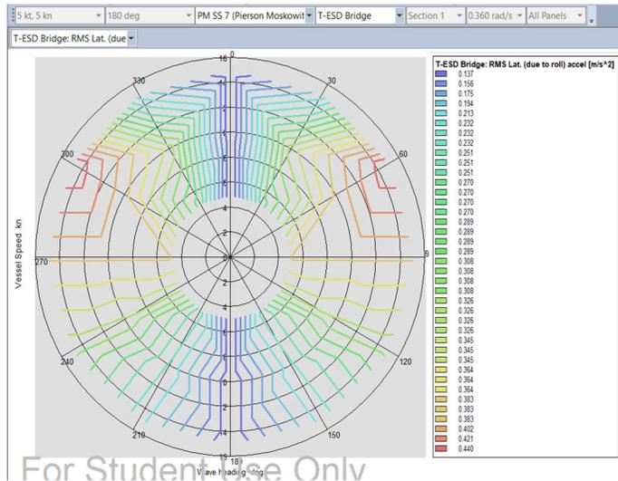
*Athwartships ship acceleration ship motion analysis for loaded vessel in Sea State 7 with max value of 0.44 g, validating the 0.49 g calculated using equations in DOD-STD-1399-301A and conservatively selected for subsequent analysis*
