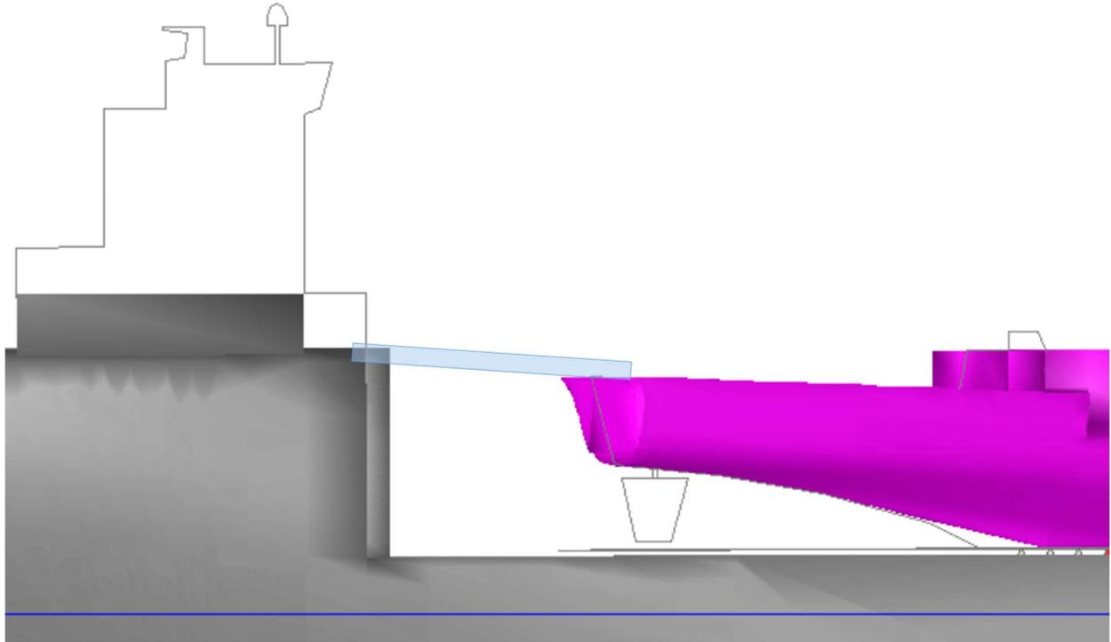
*Brow connecting Montford Point's upper deck to the target cargo's flight deck enables flow of personnel, equipment, and services*
