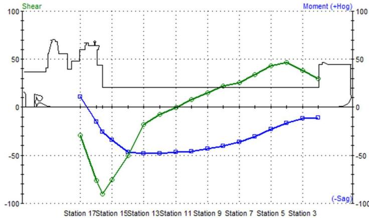
*9 m submergence percent allowable shear and moment from ballast plan*
