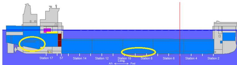
*Profile view of 9 m submergence with distributed fixed ballast*
