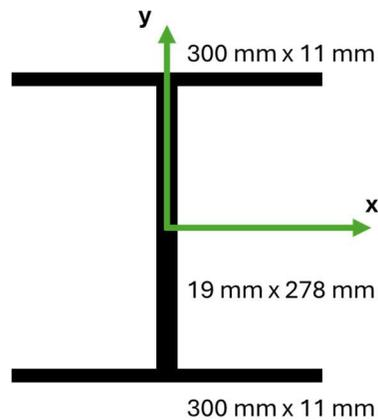
*I-beam geometry and dimensions for spur shore design*
