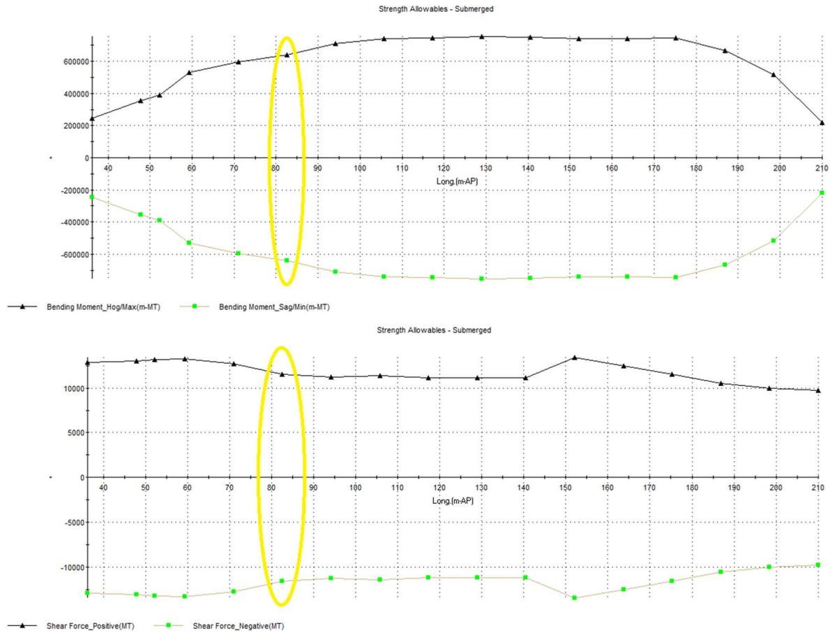
*Strength allowables with propeller pit cuts in station 13*
