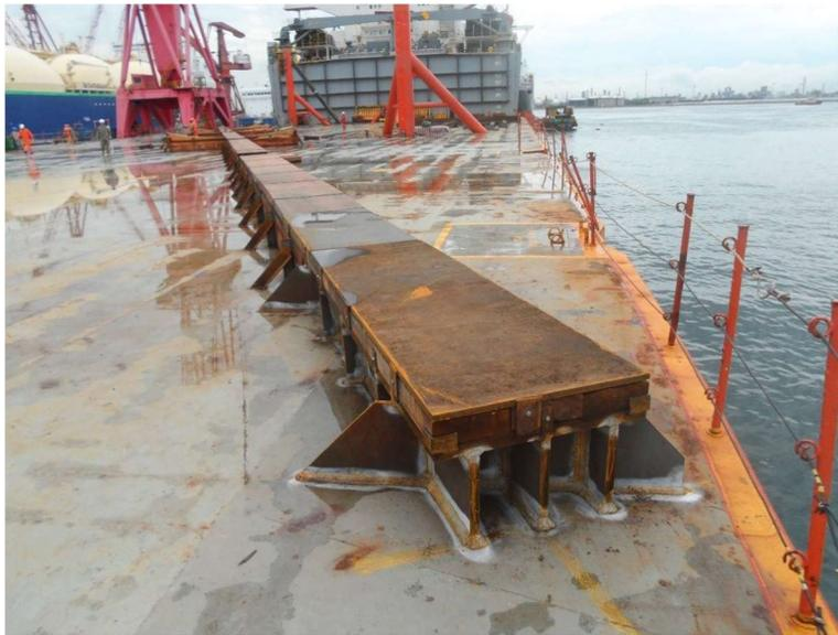
*Keel block arrangement with steel cap over soft wood used for transport of USS John S. McCain (DDG 56) aboard MV Treasure*
