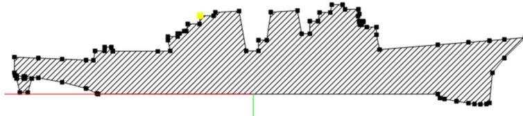
*POSSE model used to determine cargo's cross sectional area presented to beam winds and moment arm from Montford Point's Deck to center of projected area*
