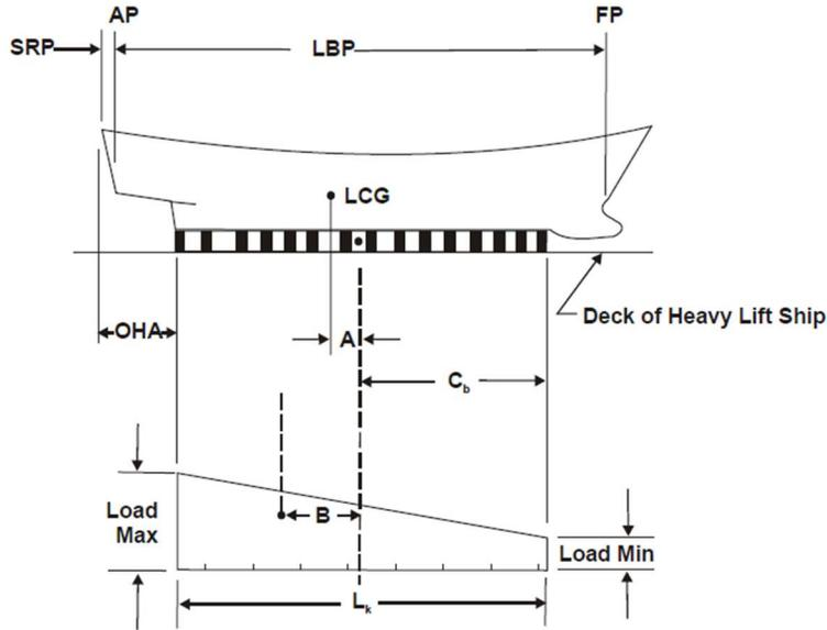
*Graphical representation of weight distribution using trapezoidal approximation method*
