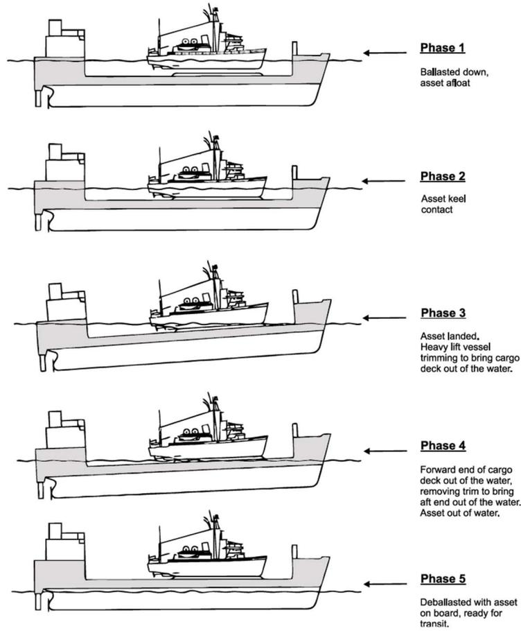
*Five phases of stability for a heavy lift drydocking*
