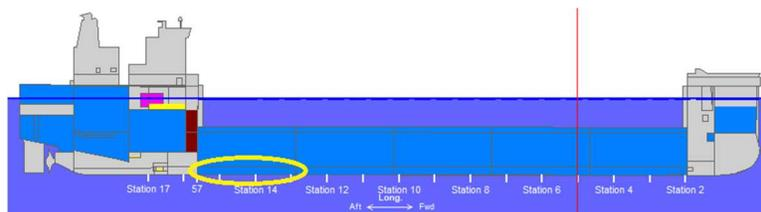
*Profile view of Montfort Point at 9m submergence with fixed ballast locations per ballasting plan identified*
