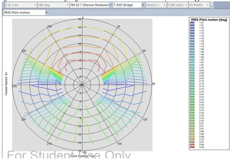
*Pitch ship motion analysis for loaded heavy lift vessel in Sea State 7 (3 degree max pitch angle)*
