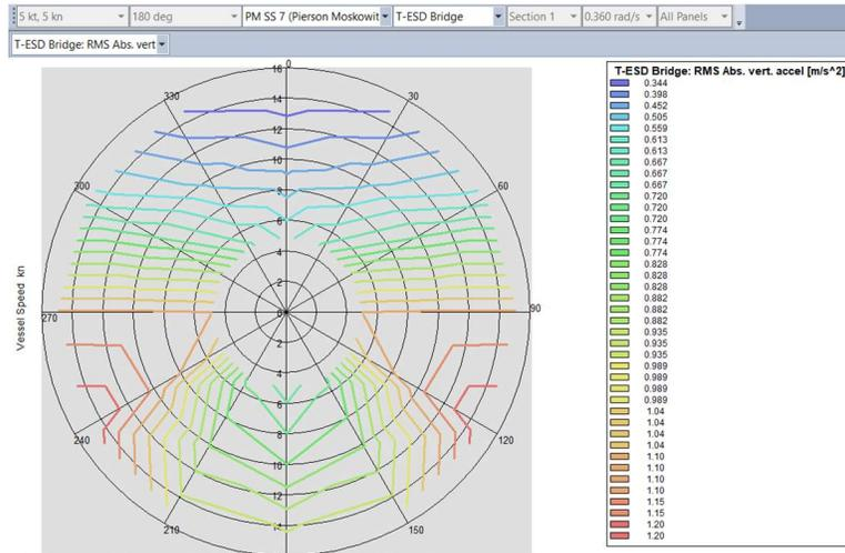
*Vertical ship acceleration ship motion analysis for loaded vessel in Sea State 7 with max value of 1.20 g, validating the 1.38 g calculated using equations in DOD-STD-1399-301A and conservatively selected for subsequent analysis*
