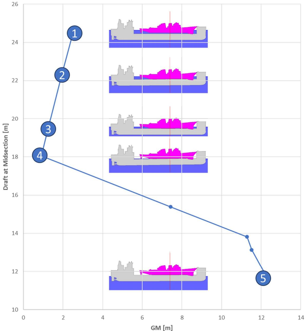
*Representative sampling of data points used to monitor evolution of GM throughout docking evolution. A minimum GM of approximately 1 m occurs during phase 4 when the waterplane area is lowest.*
